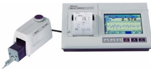
Figure 4. Stylus Surface Roughness Apparatus
